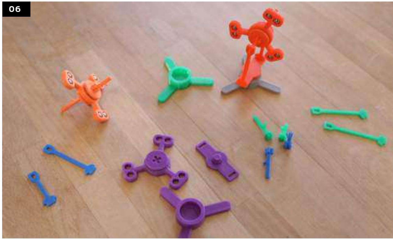
Record how long the spinner spins before stopping completely for each change in height, be sure to observe the movement of the spinner as well as that of the rotor.
