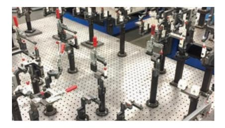
at a fraction of the cost. The fixtures could be printed and then used the next day on the welding table - and with minimized setup time, as each fixture is customized for its specific application. This provided a favorable contrast to using modular welding fixtures, which are imprecise and require additional time for adjustments to fit exact needs.
