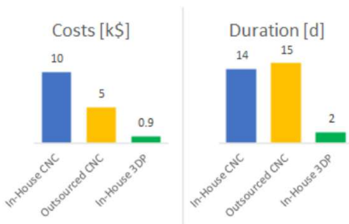
LEAD TIME AND COST COMPARISON FOR A CMM JIG AT NIKOLA CORP.
