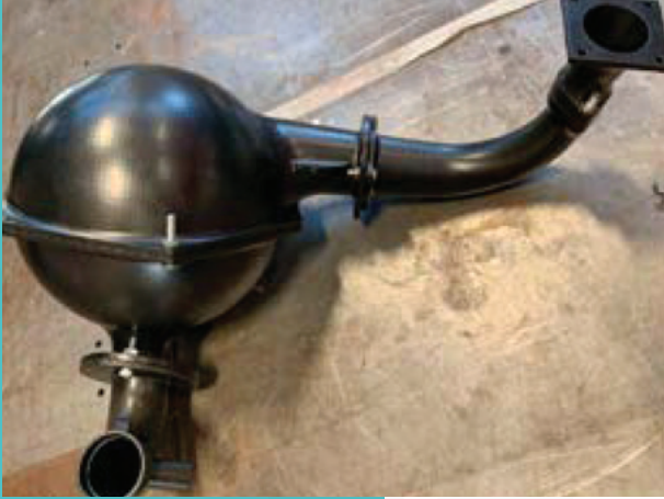
The completed plenum assembly.
