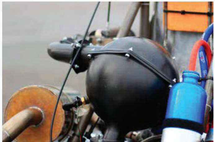
The plenum printed in Onyx on the Markforged X7 by GoPrint3D.
