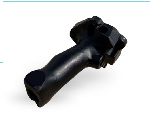
Post-processed part after impact test
