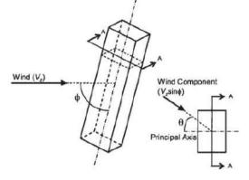
The member orientation angle,  $\theta$ , is defined as the angle in degrees between the wind component acting perpendicular to the longitudinal axis and the principal axis of the member, with the principal axis normal to the longitudinal axis. The angle  $\theta$  lies in a plane normal to the longitudinal axis, and is used to select a shape coefficient per 8.3.3.4. For wind walls,  $K_i$  equals 1.0.
