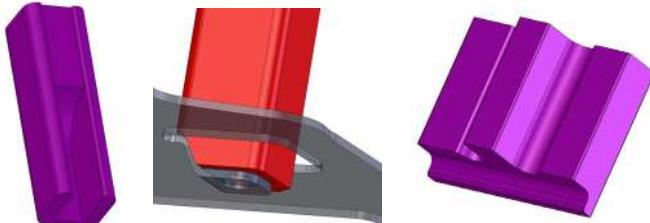
If later on you decide to create an **insert** around your punch or die mounting, Logopress3™ offers you a dedicated feature to do this very easily, including the ability to automatically create a shim under the insert.
