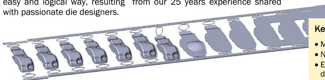
The Logopress3™ strip module can be started from a blank and a folding/stamping process that was first defined using the Logopress3™ Unbending and Flattening tools or from dumb imported data provided by your customers or partners.
