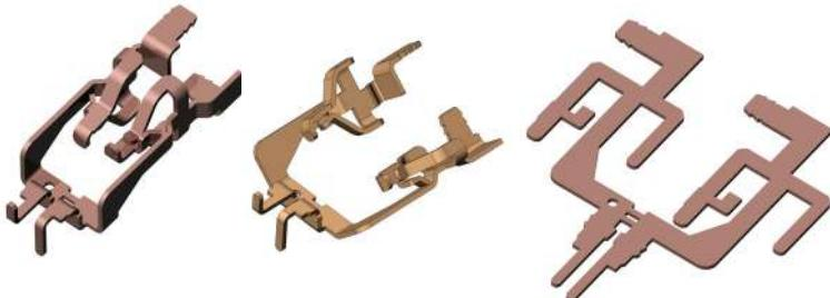
The K-Factors for each individual bend can be automatically calculated by Logopress3™ and the unfolding/unbending features can very easily be edited. This way, you can switch from a full unbending to a partial unbending. You can change the partial unbending angle value, you can manage the spring back options, the bend allowance, etc.
