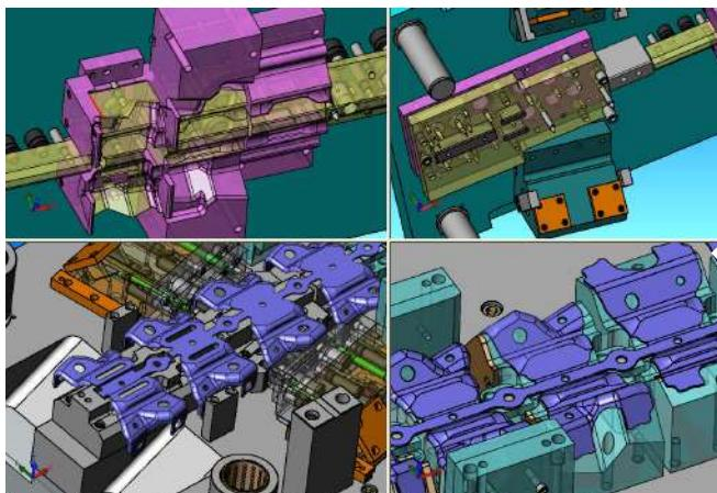
No die design software is complete unless it has a thorough **Intelligent Standard Component Library**. The Logopress3™ library not only inserts the component you select but also cuts every hole in each plate and automatically manages all mates.
